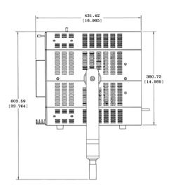
LED, 5600K CCT, 92+ CRI Passive/Active Junior Pin/28mm Spigot ETL, UL, CSA, CE and RoHS Compliant
